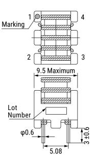
Pin Pattern Gauge Dimensions - Millimeters Tolerance ±0.1 mm
