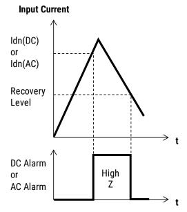
When the residual current exceeds the threshold level (Idn(DC) or Idn(AC)), PIN 4 (DC Alarm) or PIN 5 (AC Alarm) will change from low level to high impedance. Each output goes back from high impedance to low level when residual current falls below recovery level.
