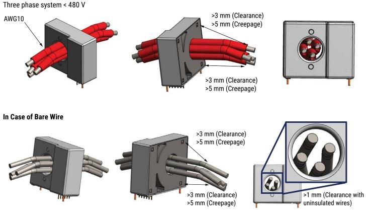
Reinforced insulation, insulation material group III, pollution degree 2, altitude < 5,000 m and overvoltage category II. Please take enough creepage distance between each pin.
