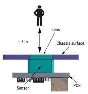
A lens is required to detect up to 5 m.
