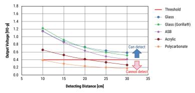
Measuring conditions: Transfer velocity - 1 m/s
