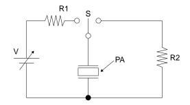
Protective resistor R1=1k $\Omega$ Protective resistor R2=1k $\Omega$ Polarizing conditions: DC voltage application  $0V\rightarrow150\pm0.2V$  (to be retained for 10 seconds)  $\rightarrow0$
