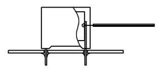
Temperature monitored inside the capacitor.
