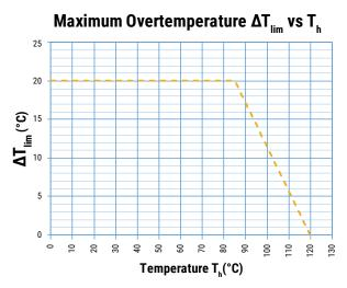
$T_h$  is the maximum ambient temperature surrounding the capacitor or hottest contact point (e.g. tracks), whichever is higher, in the worst operation conditions in °C.
