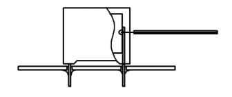
Temperature monitored inside the capacitor.
