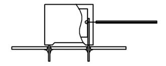
Temperature monitored inside the capacitor.
