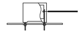
Temperature monitored inside the capacitor.
