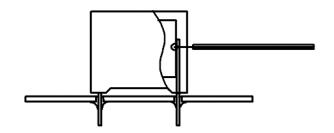
Temperature monitored inside the capacitor.
