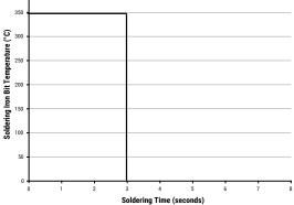
Soldering iron tip temperature should be set at 350°C (+10°C maximum), with the soldering duration not to exceed 3 seconds.
