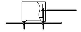
Temperature monitored inside the capacitor.
