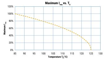
*T<sub>h</sub>* is the maximum ambient temperature surrounding the capacitor or hottest contact point (e.g. tracks), whichever is higher, in the worst operation conditions in °C.
