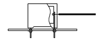
The temperature is monitored inside the capacitor.
