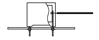
Temperature monitored inside the capacitor.
