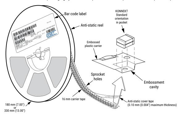
Table 4 - Carrier Tape Configuration, Embossed Plastic (mm)
