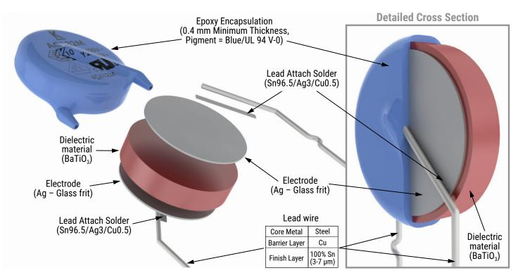
Radial Leaded Ceramic Disc Capacitors Safety Standard Recognized, C900, Encapsulated, AC Type, X1 400 VAC/Y2 250 VAC (Industrial Grade)
