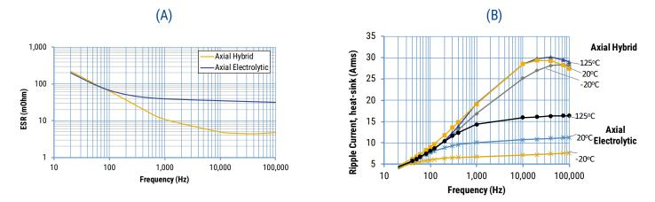
Frequency dependencies of ESR measured at 20oC and 100 kHz for Axial Hybrid (PHA225MKP3370QE4) and Axial Electrolytic (PEG226MG3370QE1) capacitors (A); Frequency dependencies of max. short pulse Ripple Current at different temperatures for heat-sink mounted Axial Hybrid (PHA225MKP3370QE4) and Axial Electrolytic (PEG226MG3370QE1) capacitors (B).
