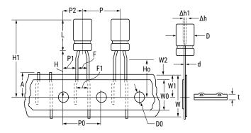
Fig. 3 (Diameter for Φ6 to Φ8) 6 – 8 mm EA
