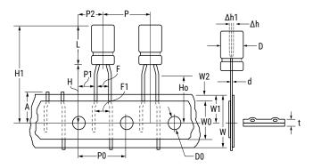
Fig. 3 (Diameter for Φ6 to Φ8) 6 – 8 mm EA
