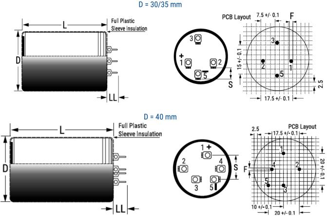
Connections: Hole 1 represents +ve. Hole 5 Represents -ve. Terminals 2,3, and 4 may be at negative terminal potential due to the presence of electrolyte. They are intended for mechanical connections only. It is recommended that they are soldered to the printed cicuit board. Additional dummy pins are provided for stability. Note that the case and dummy pins may be at negavtive terminal potential
