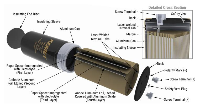
Screw Terminal Aluminum Electrolytic Capacitors - ALS42/43, +105°C
