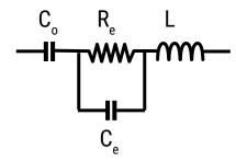
C<sub>o</sub> = Aluminum oxide capacitance (surface and thickness of the dielectric.)
