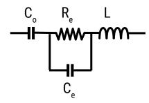
C<sub>o</sub> = Aluminum oxide capacitance (surface and thickness of the dielectric.)
